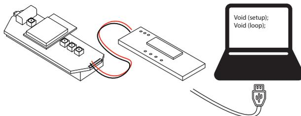
Arduino code upload through programming board
