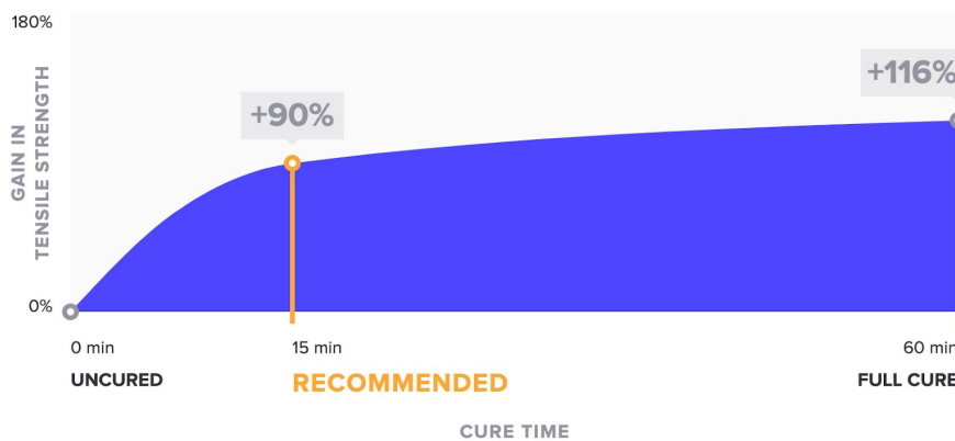
Fig. 3. Settings from the FormLabs support to cure the resin.
